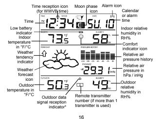
\* When the signal is successfully received by the Weather Station, the outdoor transmission icon <sup>™</sup> will be switched on. If not successful, the icon will not be shown on LCD. The user can then easily see whether the last reception was successful (icon on) or not (icon off). A short blinking of the icon indicates that signal reception is currently taking place.
